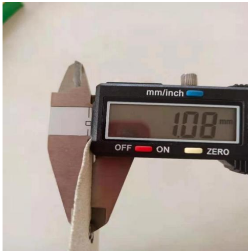
Figure 3.4 60 Baume First Pass Coating Thickness Figure 3.5 65 Baume First Pass Coating Thickness
