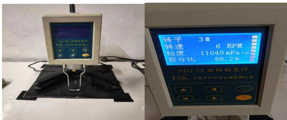
Fig. 3.3 Rotating viscometer for testing paint viscosity between Baume degree 60~65.
