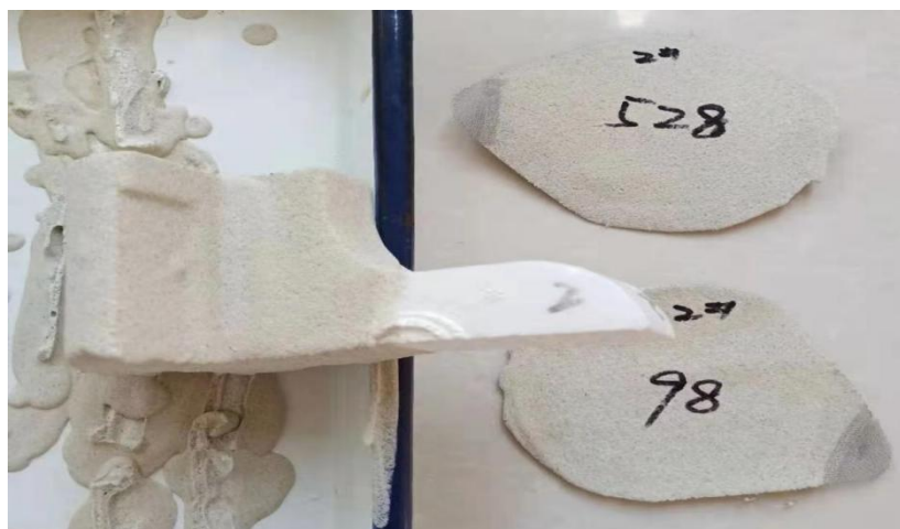
Fig. 3.10 Permeability of the coating over and over again and cracking of white mold coating.
