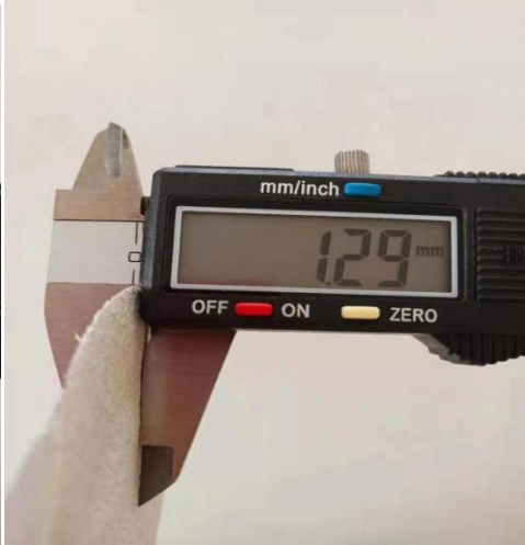
Figure 3.4 60 Baume First Pass Coating Thickness Figure 3.5 65 Baume First Pass Coating Thickness
