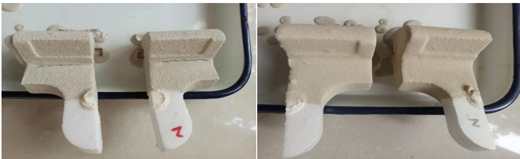
Figure 3.1 Cracking in the first pass Figure 3.2 No cracking in the second pass
