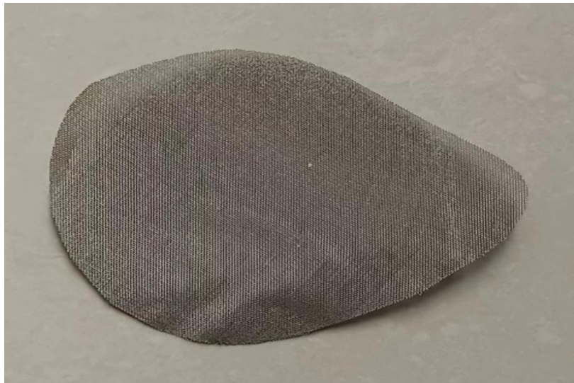
Figure 3.9 Steel wire mesh for measuring air permeability of paint once and twice.
