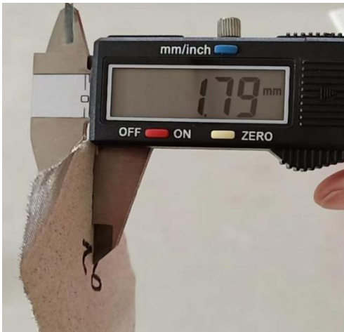
Fig. 3.6 Paint thickness of 60 Baume Second Pass Fig. 3.7 Material thickness of 65 Baume Second Pass
